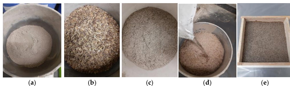
Figure 1. Fabrication of a sample with rice husk vegetal fiber: (a) Dry base formula; (b) rice husk fiber; (c) mixed compound; (d) adding water into the mix; (e) mortar into the square mold.
