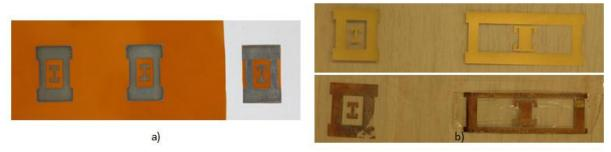
**Figure A.11.** Inkjet-printed E-plane inserts with I-shaped insets for compact waveguide filters: a) Kapton substrate, Dimatix DMP-3000 printer; b) PET substrate, Epson Stylus C88+ printer, without (up) and with (down) copper electroplating.
