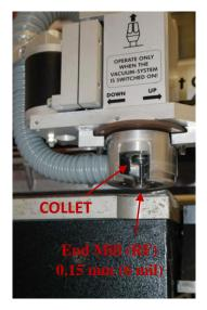
**Figure A.4.** ProtoMat C60 mill/drill head with high-speed spindle having end mill tool in its shaft.
