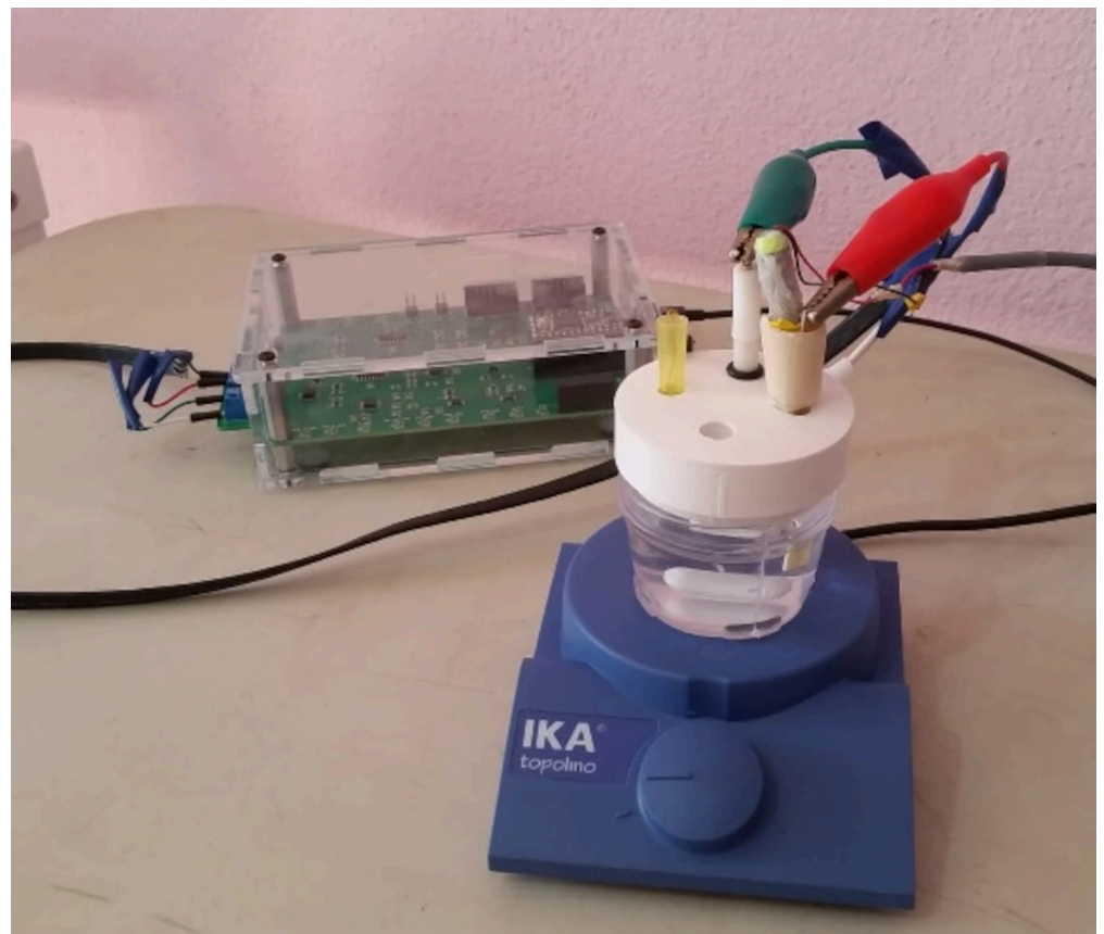
Fig 1. Low-cost electrochemical instrumentation for the detection of arsenic used in this work. In this case, the gold microwire set-up is presented. The Rodeostat potentiostat (in the transparent plastic housing at the back of the image) is connected to the electrodes via a shielded ethernet cable. The electrodes are mounted in a 3D printed plastic lid with an extra opening port for addition of the arsenic standard solution via pipette (to avoid knocking the electrode connections). The electrodes are (left) iridium wire counter electrode, (centre) Ag/AgCl/KCl (3M) reference electrode, and (right) gold microwire working electrode assembled with a mechanical vibrator. The 40 mL sample cell is positioned on top of a magnetic stirrer plate for mixing after addition of the sample and As(V) standard solution and possibly during the deposition stage (to increase mass transfer).
