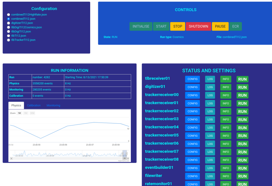
Figure 12. Example screen shot of the RCGui web application during cosmic ray data taking with the FASER detector.
