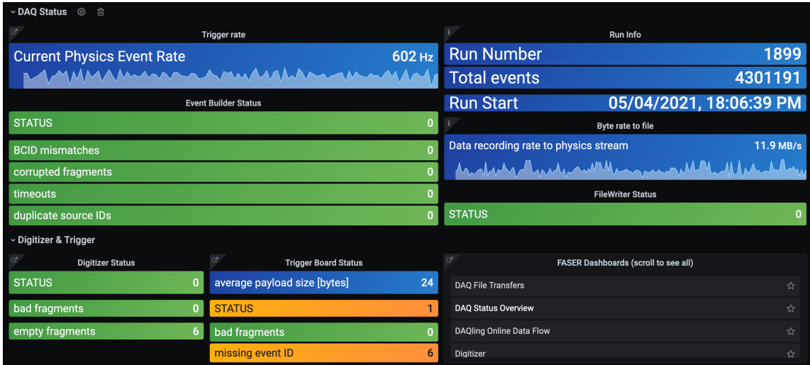
Figure 13. Grafana dashboard of the DAQ status overview for an ongoing data taking run. Metrics of the trigger and data recording rate, DAQ module status and total error counts are displayed. In addition, current run details are shown.
