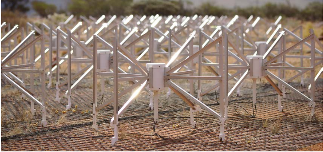
Figure 1.10. Photograph of an MWA antenna, showcasing the cross-dipole design.
