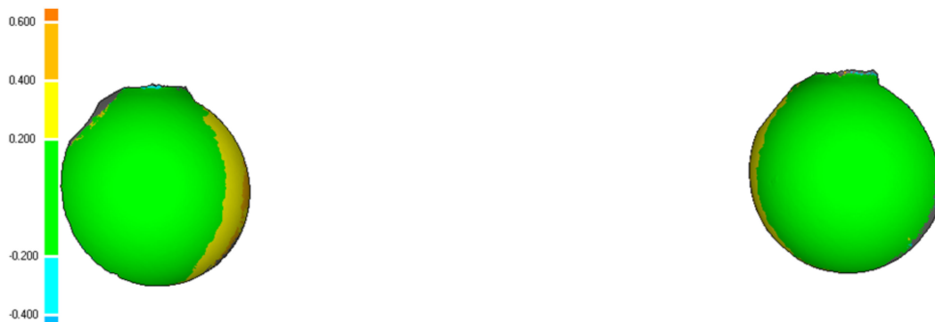
Figure 7. 3D difference image of two measurements of the ball-bed in air and water, respectively. Colors represent the deviation of the 3D coordinates (scale is in mm).
