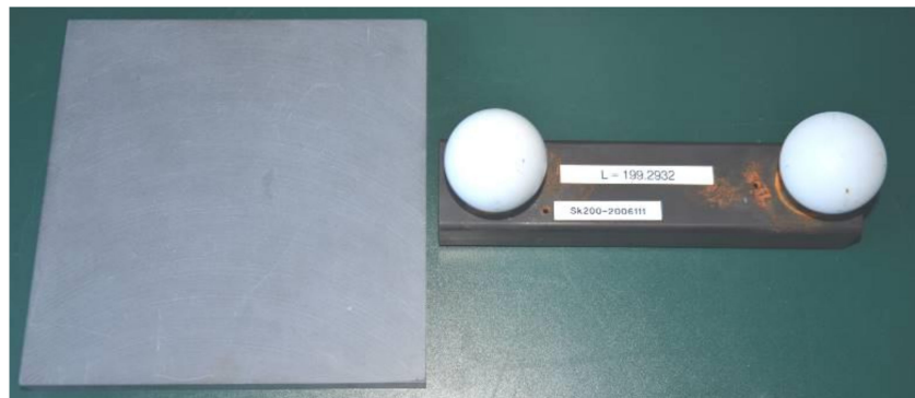
Figure 4. Measurement objects: ceramic plane (left) and ball-bed (right).
