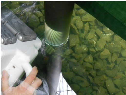
Figure 6. Projected fringe pattern during the measurement of a pipe (left) and 3D reconstruction result (right).
