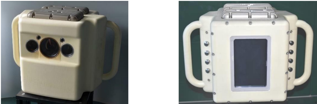
Figure 3. Handheld underwater 3D scanner, front view (left) and back view (right).
