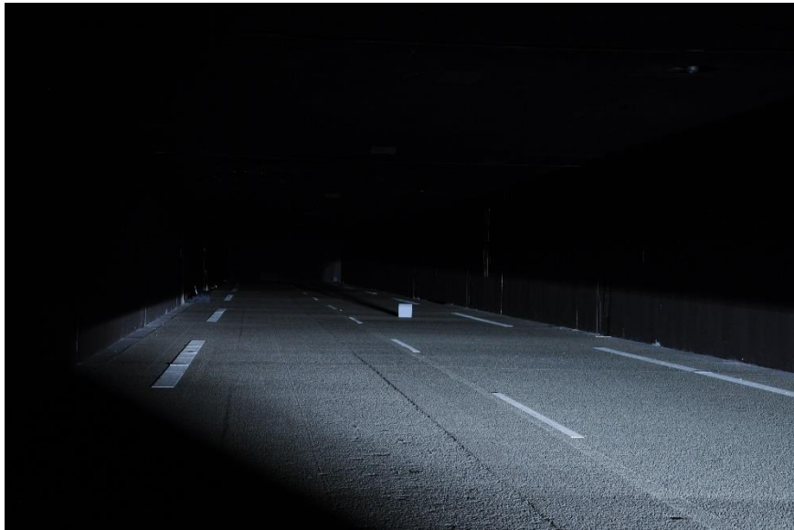
Figure 3: Grey square board with a size of 30 cm and a reflectivity \rho of 5.2 %, positioned 50 m ahead of the test persons in the middle of the driving lane served as the viewing target.
