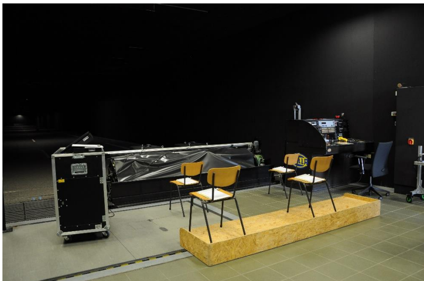
Figure 1: Study setup in the light tunnel, 4 test persons were positioned next to each other behind the video projectors looking along the road at the viewing target.
