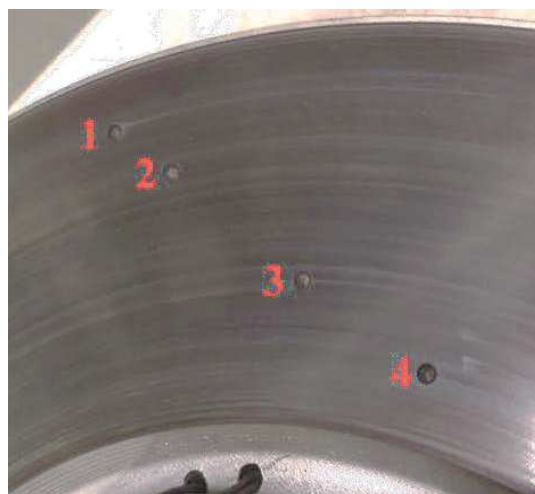
Figure 1. Position of thermocouples 1–4 on the outboard side of the disc.
