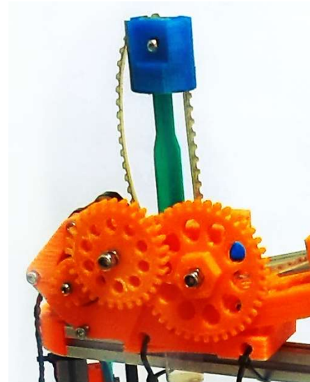
Figure 3-7. Universal paste extruder (Richard Horne). A motor turns a gear chain which pulls a toothed belt around a pulley. The belt contracts, bringing in a syringe holder, and with it depressing a syringe.
