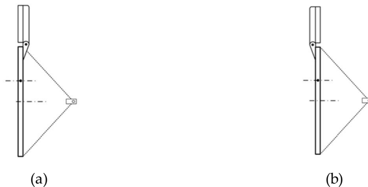
Figure 2.43 – Keying flap designs: (a) flap rotates outward; (b) flap rotates inward (Tian et al., 2014).
