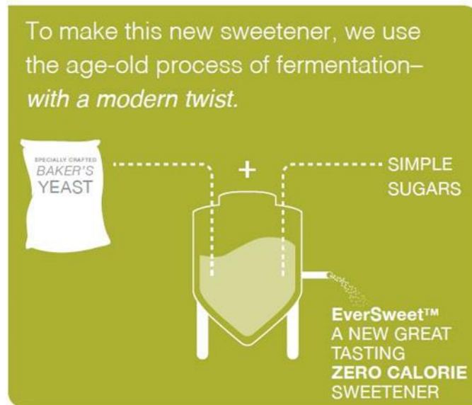
Figure 3.7 EverSweet® production process ‘info graphic’ (Cargill 2021c)
