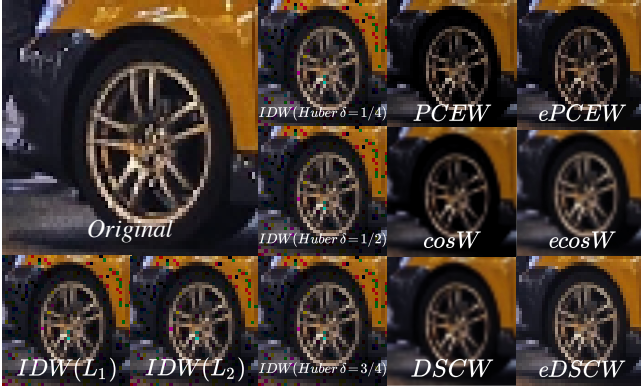
Fig. 5. Instances of average distance/similarity weighting methods. Kernel weights are determined based on IDW [12] with various inverse distance functions. Alternatively, weights are found based on similarity measures using the inner product (( e )PCEW, ( e )cosW and ( e )DSCW).
