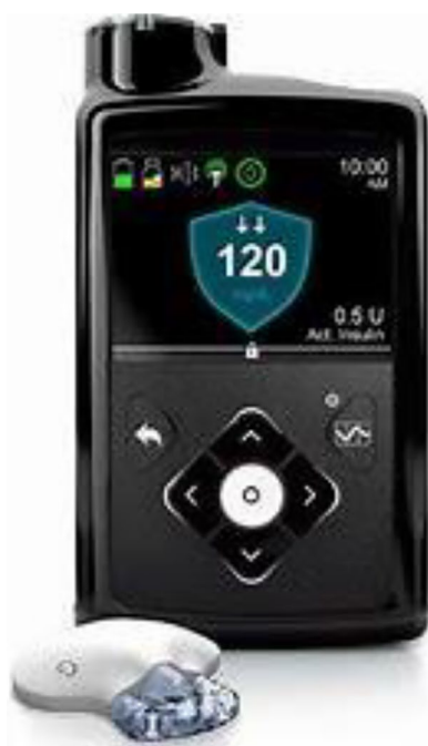
Figure 4. The Medtronic 670G with a guardian 3 sensor; an example of a hybrid closed-loop pump system.
