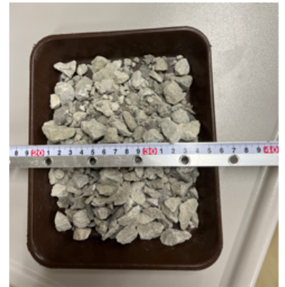
Photo of the excavated dolerite. It contains geogenic arsenic
