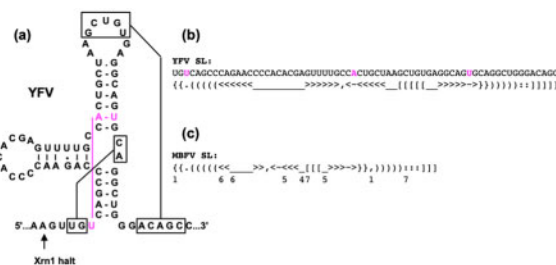
Fig. 2. An example of WUSS representation of RNA structure containing pseudoknots and a triple base interaction. (a) The structure of Xrn1-resistant stem-loop RNA structure (xrRNA) of yellow fever virus (YFV) according to the general model (MacFadden et al. , 2018). Paired regions in pseudoknots are boxed, triple base interaction is shown in magenta. The point of Xrn1 halt (Silva et al. , 2010) is indicated by arrow. (b) Structural annotation of the YFV SL domain using WUSS symbols. Dot and tildes indicate a triple base interaction. (c) The general descriptor for MBFV xrRNA SL domains. A number below a symbol in the descriptor indicates potential multiplication of the symbol in the searched structures. For instance, 5 below a symbol for base pair means that at this site 0, 1, 2, 3, 4 or 5 base pairs are allowed
