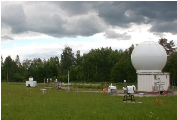
Figure 6: The radar field in Hyytiälä station: The C-band radar is the biggest one, the Ka-band radar to the left and the W-band radar is in front. Photo credit: Matti Leskinen.
