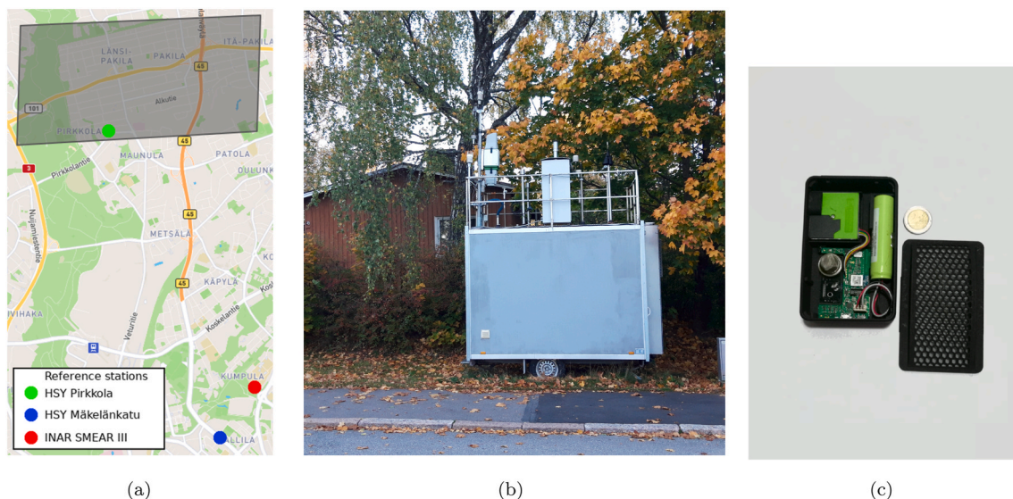
Fig. 1. (a) The districts of Pakila and Pirkkola in Helsinki are shown in the grey area. The HSY reference station in Pirkkola is shown with the green dot. (b) The HSY reference station in Pirkkola and (c) low-cost sensors used in our Pakila campaign.
