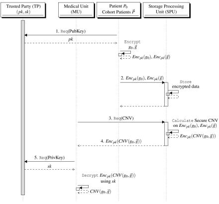
Figure 1: Message flow for a secure processing in our scenario
