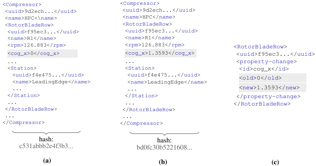
Fig. 21 XML SERIALIZATION, HASHING AND DIFF OF TURBO COMPONENT DATA RECORD
