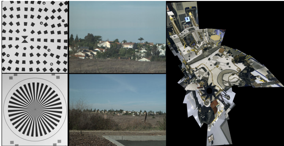
Fig. 9 Examples of characterization and calibration images taken by the flight Mastcam-Z cameras during pre-launch testing in 2019 and 2020. (Upper left) Part of an MTF test target imaged at 100 mm focal length from a range of 7 m. The central “bow tie” feature is 5.6 cm tall; (Lower left) Part of a 57-cm diameter “Siemens star” MTF test target imaged at 34 mm focal length from a range of 5 m. (Upper and lower middle) Examples of distant targets imaged at 26 mm and 110 mm focal lengths. The houses on the top of the distant ridge are approximately 1 km away. (Right) Example 34 mm focal length 360° downward-pointing mosaic of the Perseverance rover’s deck, assembled from 53 individual 34 mm focal length images taken during ATLO testing at KSC in March 2020 for geometric mapping and RSM pointing verification
