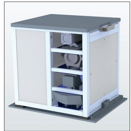
Abb. 4: Vehicle Sensor Unit (VSU-Box), Montage an beiden Spitzen der Rangierlokomotive
