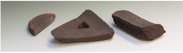
Figure 1. : Examples of 3D printed parts obtained by solar sintering of regolith simulant.
