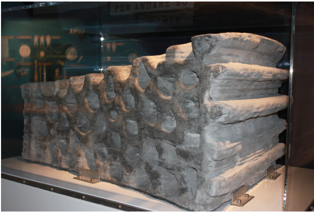
Figure 2. : Lunar habitat outer shell building block demonstrator produced by the D-Shape additive manufacturing process, using MgCl binder and lunar regolith simulant.
