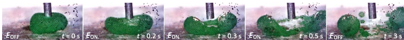
Figure S4. An electrode inserted into the PE particle covered silicone oil droplet ( \sim 2 \text{ mm} ). High electric tension ( \sim 1 \text{ kV} ) applied to the electrode caused the droplet to violently break apart.
