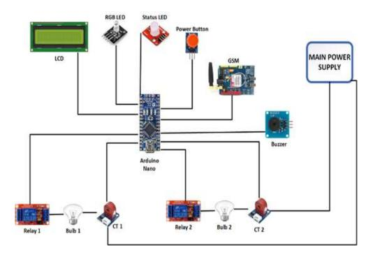
FIGURE 7. Proposed IMCB System Test Diagram
