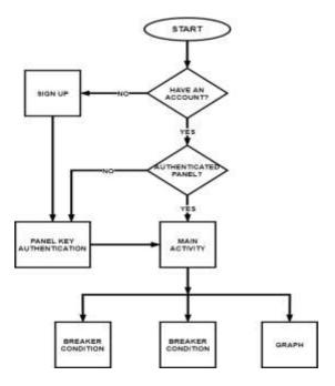
FIGURE 5. IMCB Software Application Activity Diagram
