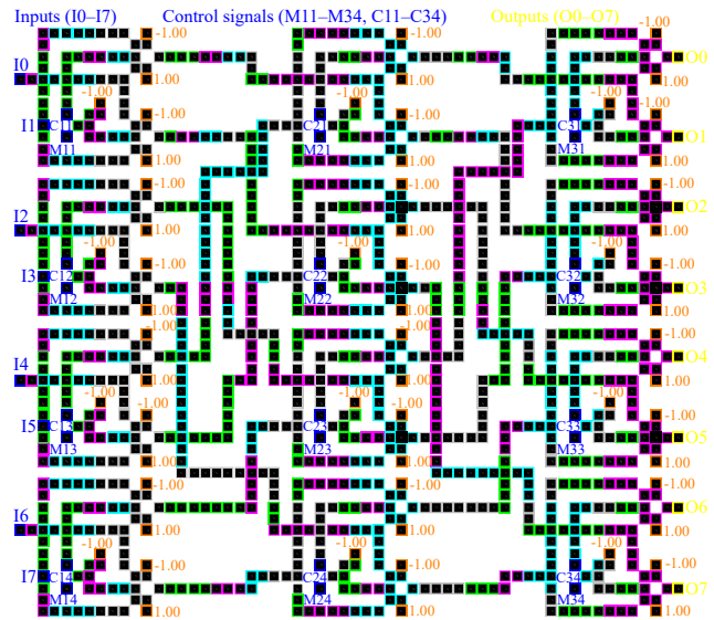
Fig. 9: QCA Schematic for 8 \times 8 M-SEN network.
