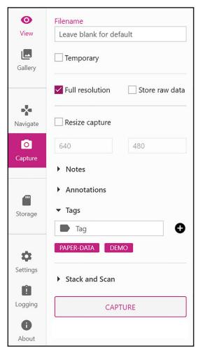
Figure 3. An example side pane from the OpenFlexure Connect microscope client. Using a web API for instrument communication allows the client to be written in any programming language. Using javascript we were able to create a cross-platform, responsive, and modern user interface using general purpose user interface frameworks.
