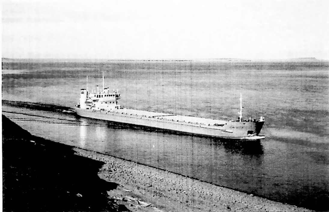
Figure 4.10 Supplies to Sakha's far north. One of the latest generation of shallow-draught freighters, the '60 Years of the Yakut ASSR', in the Lena delta, heading for Tiksi and the Yana delta. Note its proximity to the shoreline. In late summer, the navigation channel in the Lena delta becomes very shallow indeed. Source: author's photograph.
