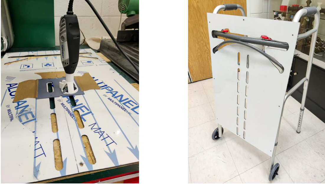
Figure 2.13: Cutting the slots for straps (left) and finished front plate on the walker (right)
