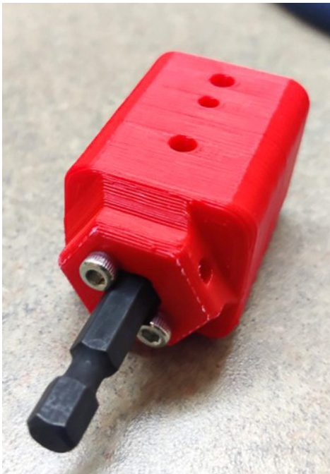
Figure 2.15: Adapter with embedded hex bit for connecting drill and square rod
