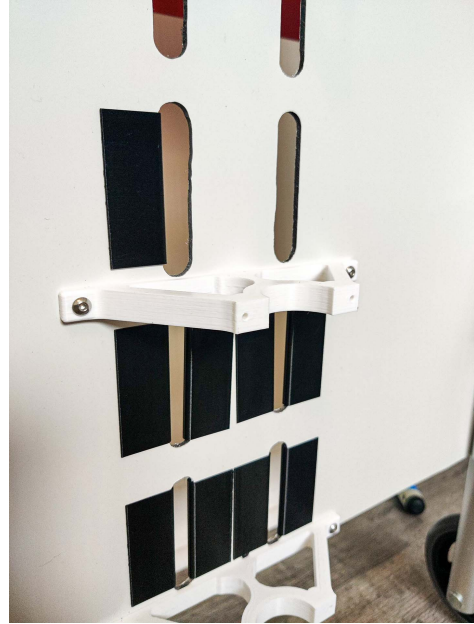
Figure 2.14: Smooth guides for the webbing straps on the 3D printer (left) and partially installed on the front plate (right)
