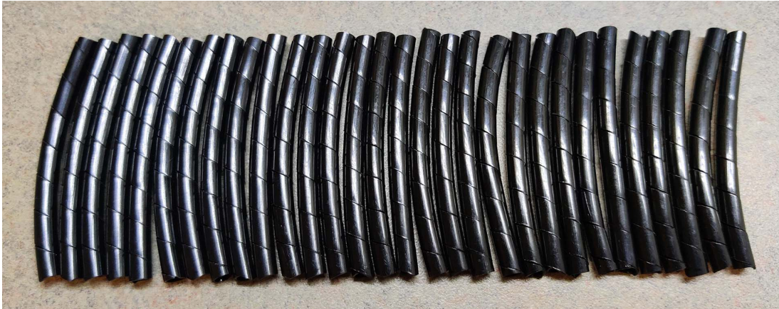
Figure 3.8: Spiral cable wrap spacers
