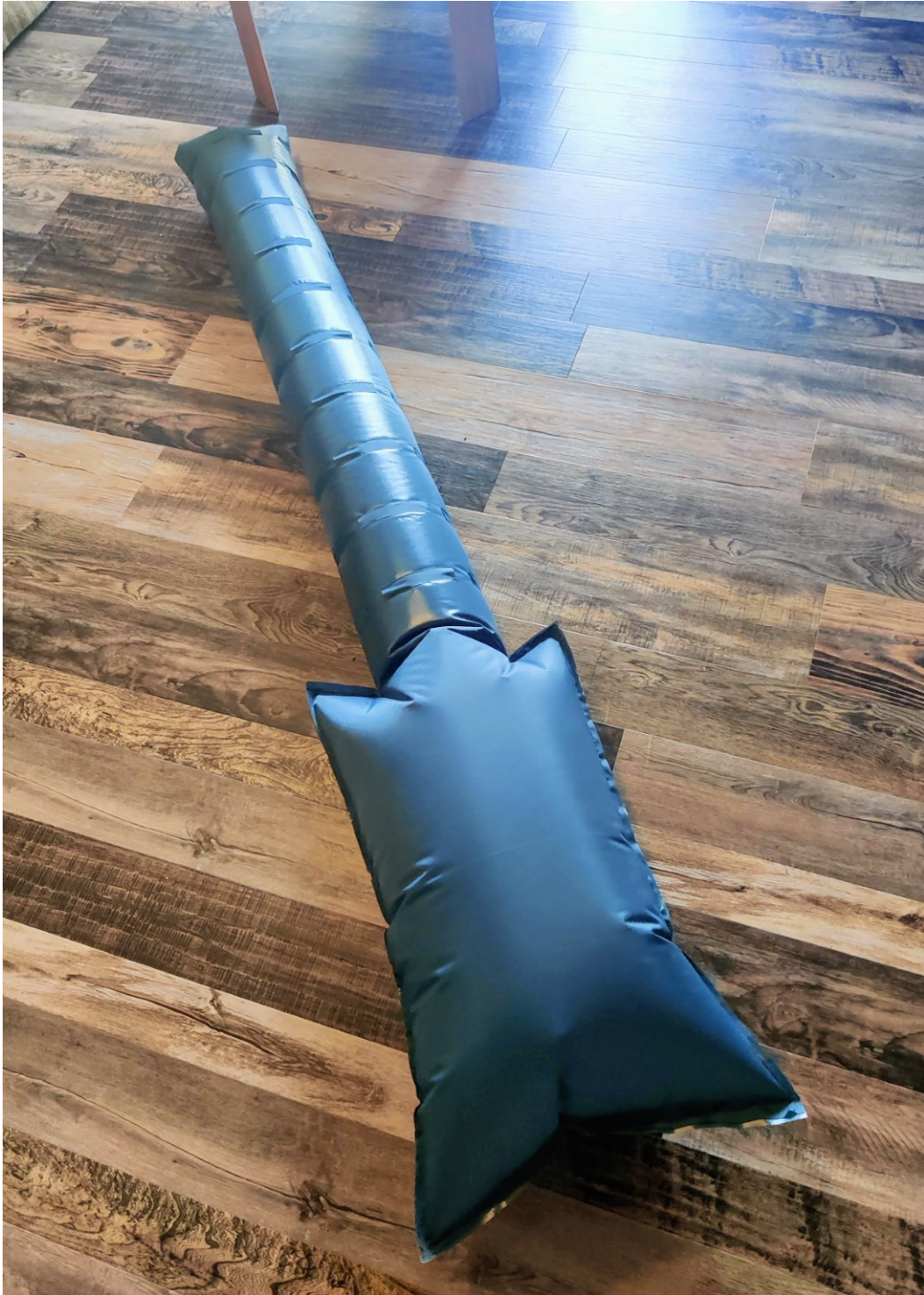
Figure 2.9: First full inflation of the fabric arm and air bladder
