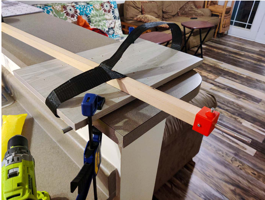
Figure 2.2: Prototype with a square rod spun by a drill
