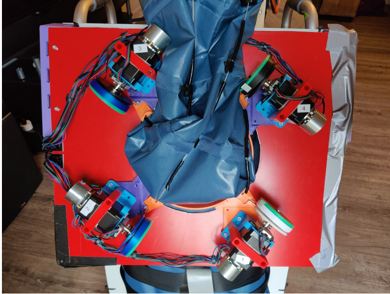
Figure 2.19: All motor assemblies mounted on the walker
