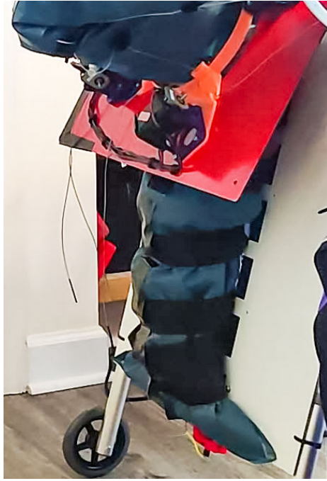
Figure 3.1: Deploy test with speed set to 2 and clutch on maximum. There is still air in the bladder that should be forced into the arm, but the drill stopped spinning before the arm was sufficiently pressurized.
