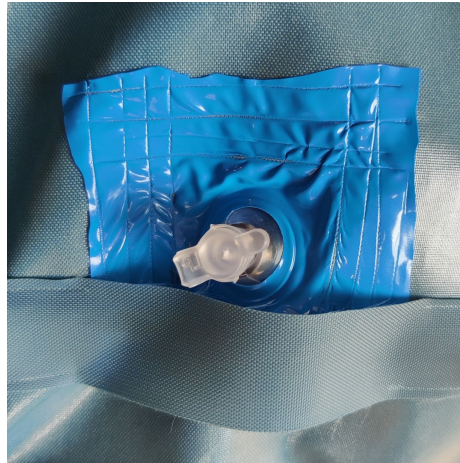
Figure 2.8: Air nozzle sealed to the arm
