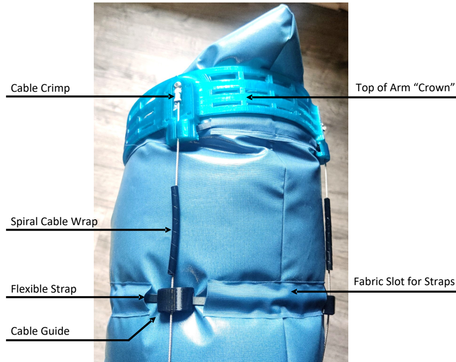
Figure 2.10: Components of the end of the arm
