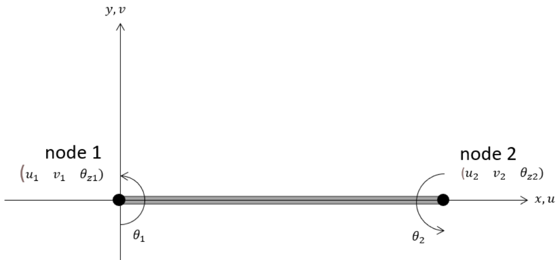
Figure 2-4 Representation of local displacements and rotations for a 2D frame element
