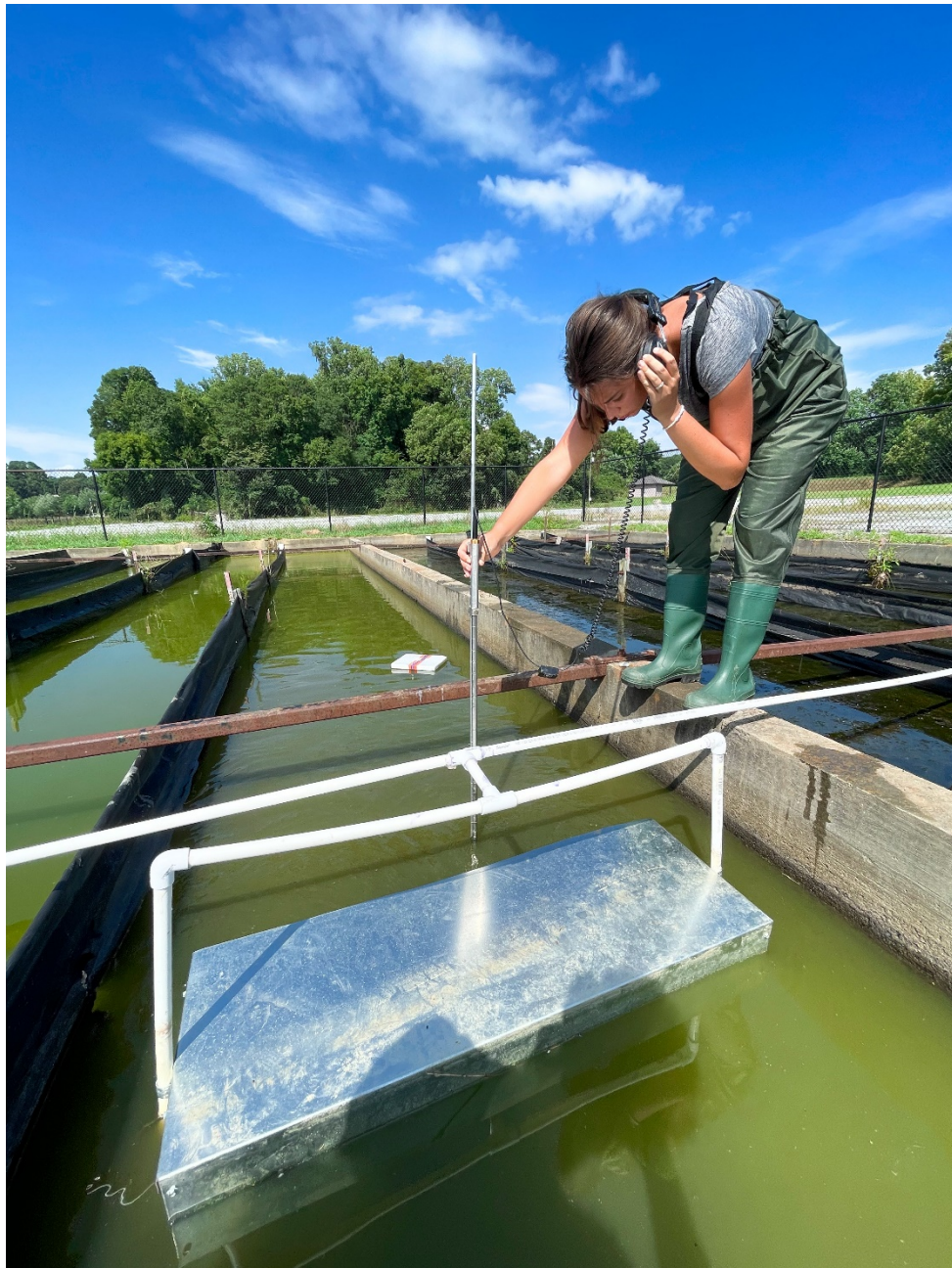
Figure 3.15: Libby Flanagan operates pygmy meter in front of airlift pump
