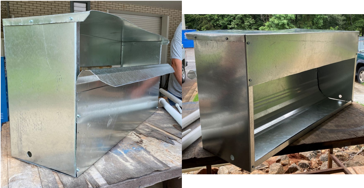
Figure 3.9: Completed Metal Assembly of Rectangular Airlift Pump
