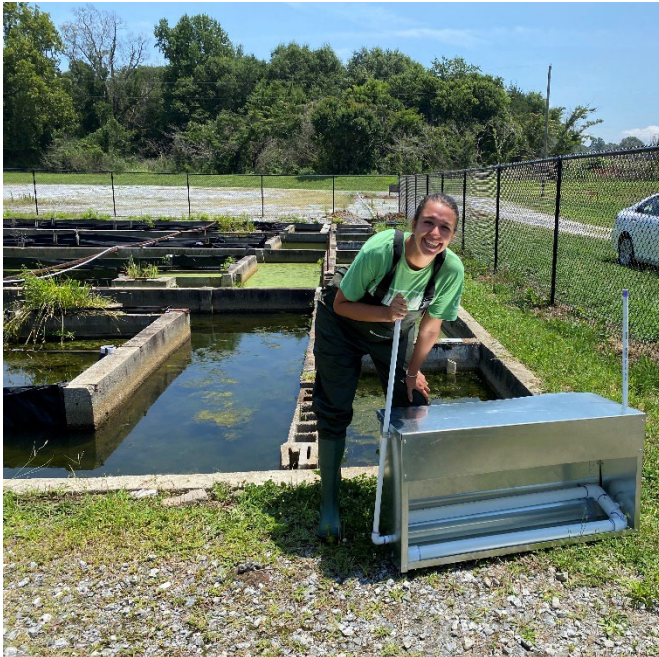
Figure 3.11: (Left) Airlift with 1/2" connection pieces before install into ACCS (Right) with full connection to 70' Long Air Distribution Line
