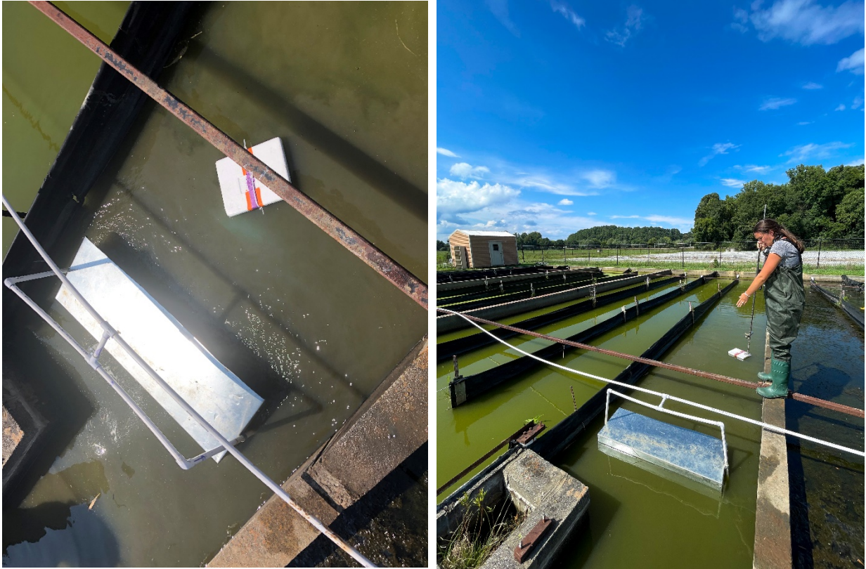
Figure 3.16: (a) Start of Drogue Test Run with visual water movement at Airlift opening (b) Middle of Drogue Test Run in Lane 1 of Raceway 3
