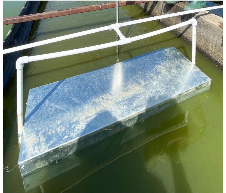
Figure 3.11: (Left) Airlift with 1/2" connection pieces before install into ACCS (Right) with full connection to 70' Long Air Distribution Line
