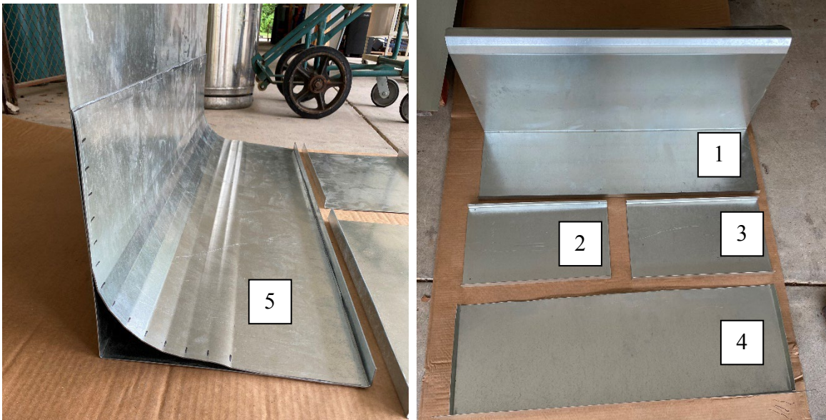
Figure 3.8: Rectangular Airlift Pump Metal Pieces for Fabrication
