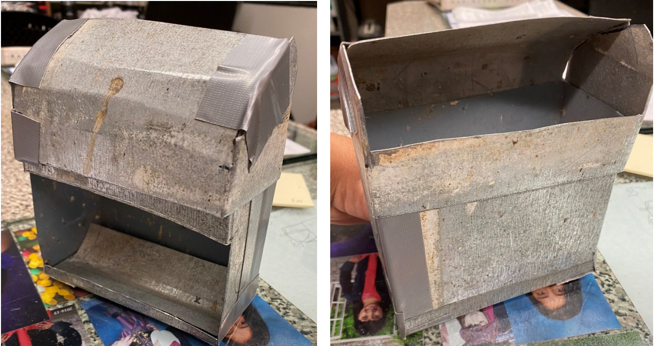
Figure 3.7: Rectangular Airlift Pump Design Prototype by Rodney Morgan
