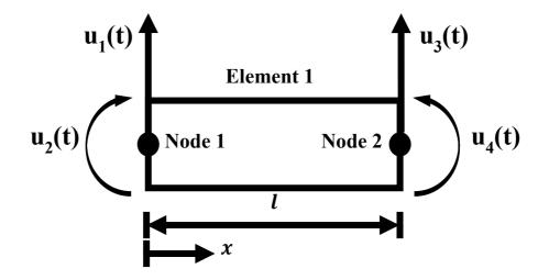
Figure 4: Element nodal displacement schematic
