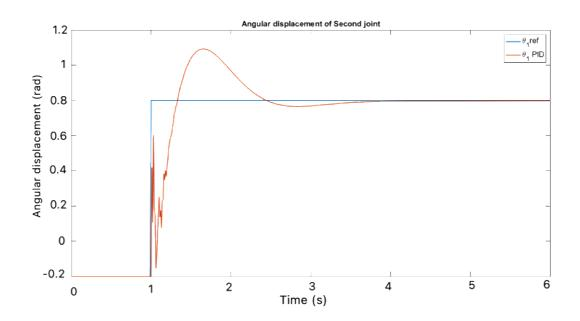
Figure 18: Angular displacement  $\theta_2$  of link 2 with PID controller
