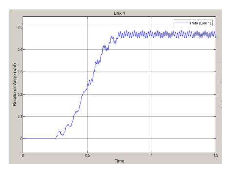
Figure 9: Rotational angle ( $\theta$ ) of link 1without a controller
