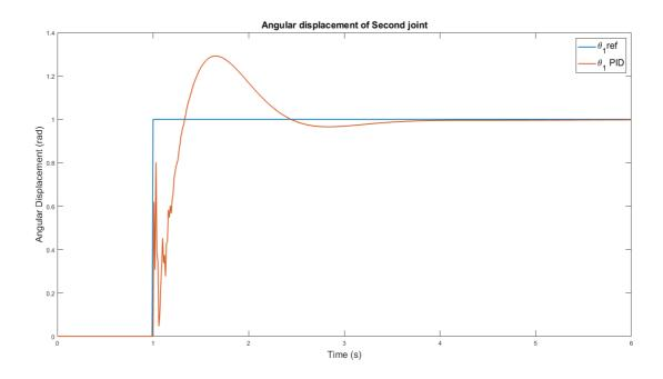
Figure 39: Angular displacement of second joint for the PID controller
