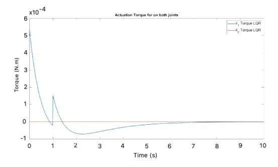
Figure 68: Actuation torque feed to both link actuators of the simulated model with LQR controller
