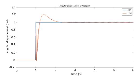
Figure 38: Angular displacement of first joint for the PID controller
