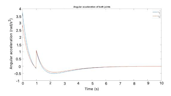
Figure 63: Angular acceleration of both joints of the simulated model with LQR controller
