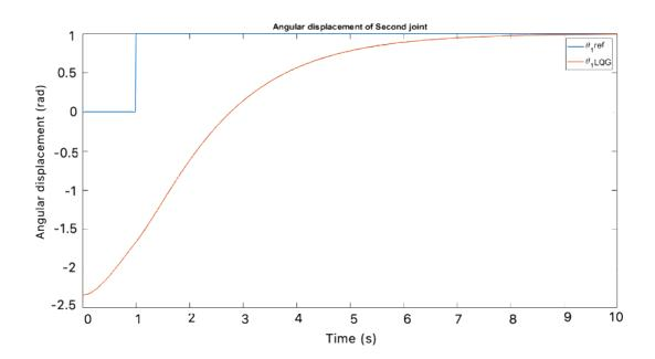
Figure 66: Angular displacement of link 2 of the simulated model with LQG controller
