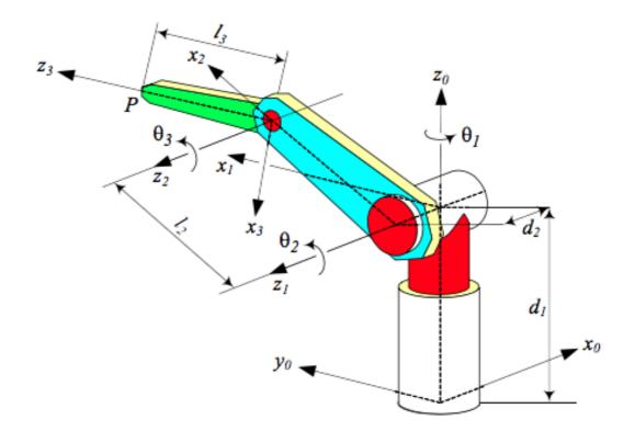
Figure 1: Schematic for three revolute joint manipulators
