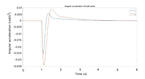
Figure 35: Angular acceleration of both joints with LQG controller
