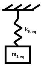
Figure 81: Equivalent simple spring mass system for link 2
