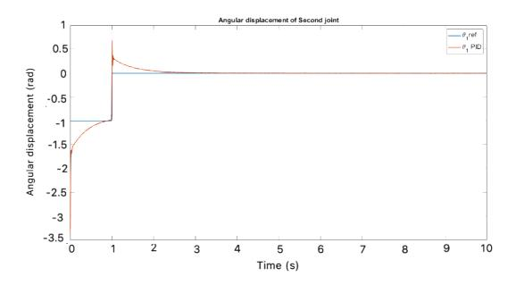
Figure 52: Angular displacement of link 2 of the simulated model with PID controller
