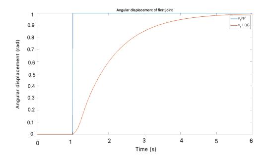
Figure 31: Angular displacement of link 1 with LQG controller
