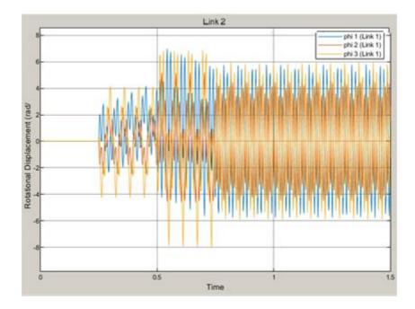
Figure 11: Rotational displacement of link 1wihtout a controller
