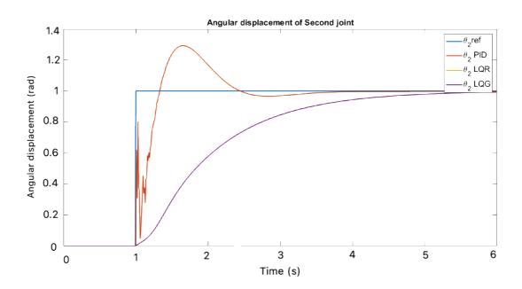
Figure 41: Comparison between angular displacement of link 2 for the three controllers
