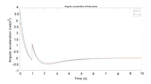
Figure 70: Angular acceleration of both links of the simulated model with LQR controller
