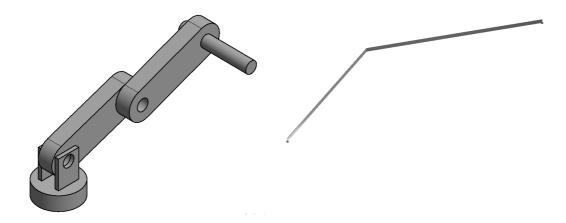
Figure 47: Two- link manipulator model in Autodesk Inventor
