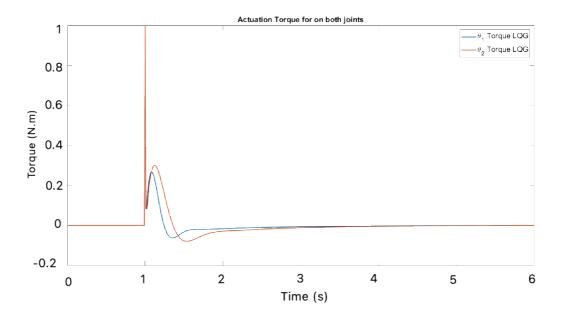
Figure 36: Actuation torque signal from the LQG controller with LQG controller
