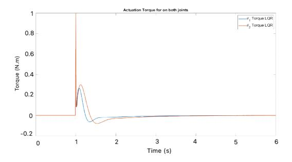
Figure 27: Actuation torque for both joints with LQR controller
