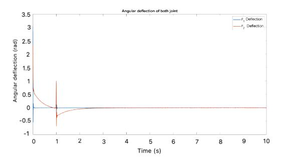
Figure 53: Angular deflection of both links of the simulated model with PID controller
