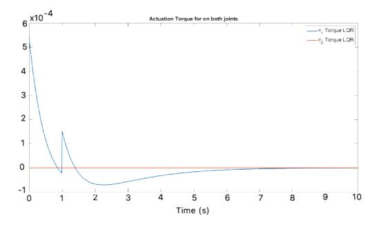
Figure 61: Actuation torque for both links of the simulated model with LQR controller
