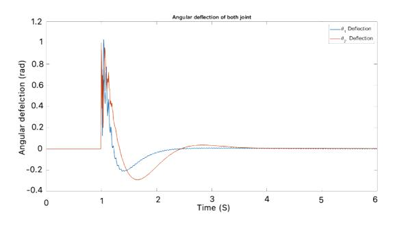
Figure 19: Deflection of nodes of link 1 and link 2 with PID controller
