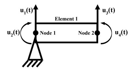
Figure 85: Element nodal displacements and constraint
