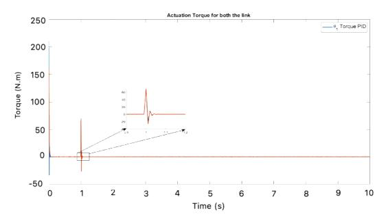
Figure 54: Actuation torque to both links of the simulated model with PID controller
