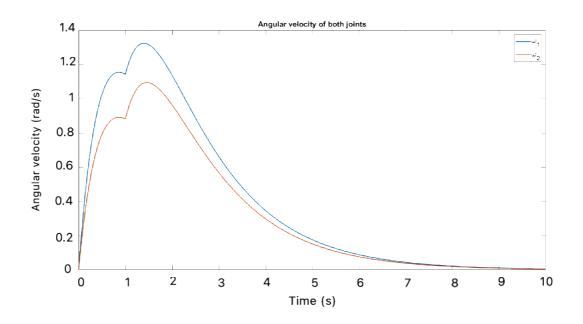
Figure 69: Angular velocity of both links of the simulated model with LQR controller
