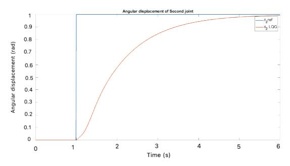
Figure 32: Angular displacement link 2 with LQG controller
