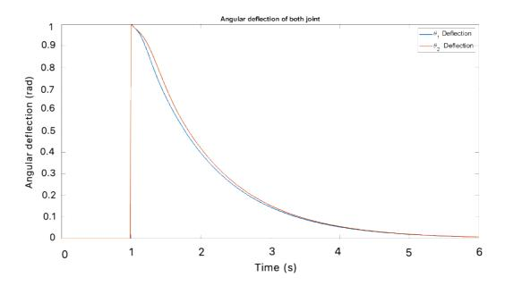
Figure 33: Angular deflection of both joints with LQG controller
