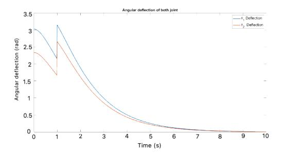
Figure 60: Angular deflection of both links of the simulated model with LQR controller
