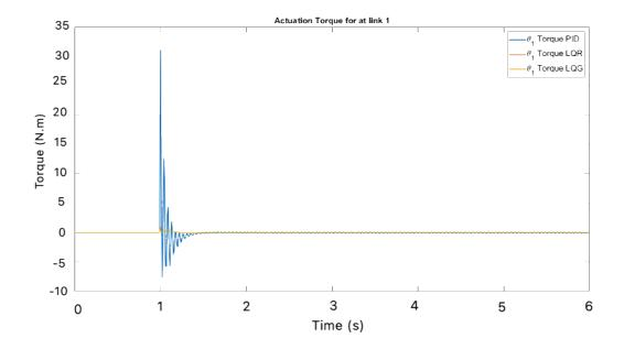
Figure 42: Comparison between actuation torque of link 1 for the three controllers
