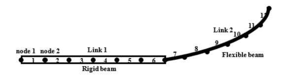
Figure 3: Beam elements for two links
