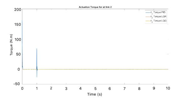
Figure 74: Actuation torque of link 2 of the simulated model with the three controllers
