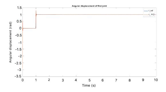
Figure 51: Angular displacement of link 1 of the simulated model with PID controller
