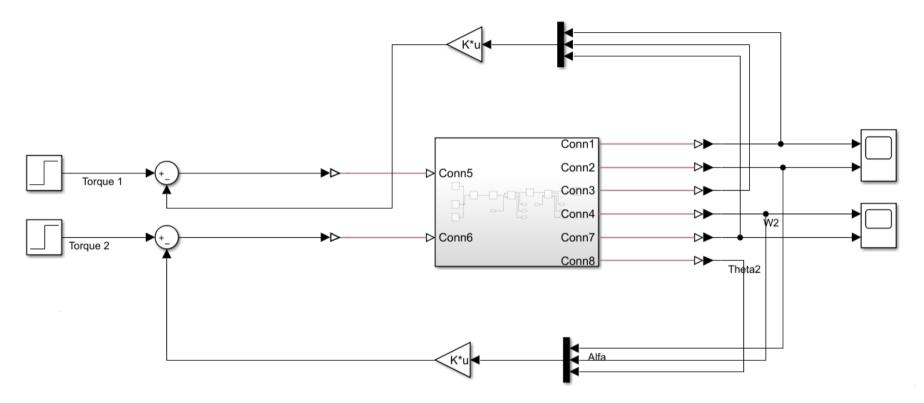
Figure 57: Simulation of two-link manipulator with LQR controller
