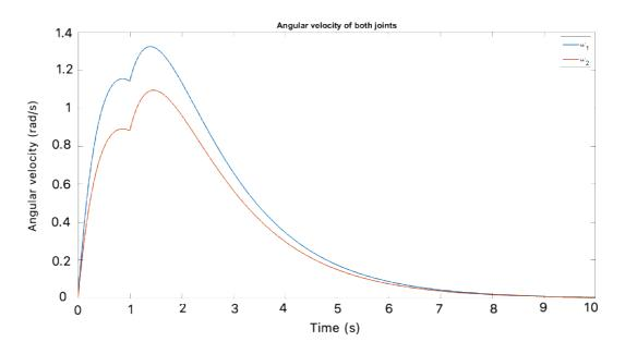
Figure 62: Angular velocity of both links of the simulated model with LQR controller
