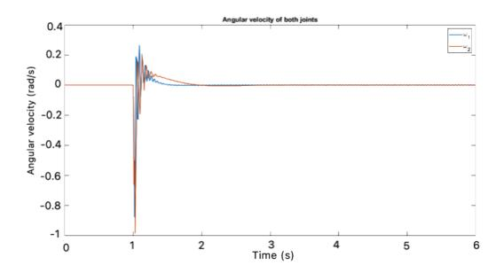
Figure 20: Angular velocity of link 1 and link 2 with PID controller
