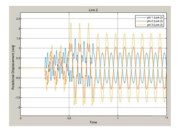
Figure 14: Rotational displacement of link 2 without a controller
