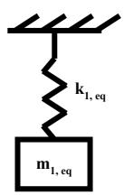
Figure 78: Equivalent simple spring mass system for link 1
