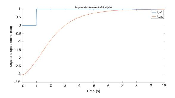
Figure 65: Angular displacement of link 1 of the simulated model with LQG controller
