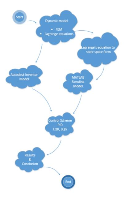
Figure 5: Flow chart of modelling methodologies
