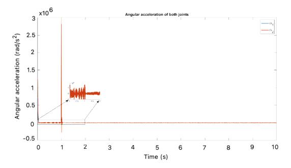
Figure 56: Angular acceleration of both links of the simulated model with PID controller
