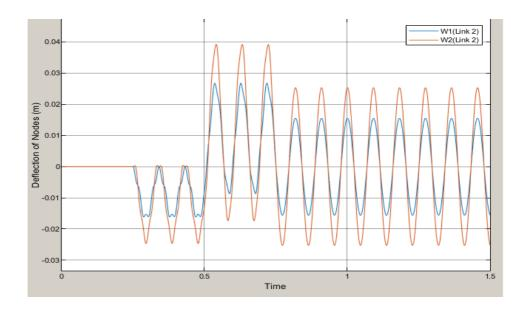
Figure 13: Deflection of nodes of link 2 without a controller
