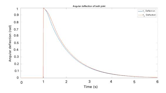
Figure 26: Deflection in both joints from the desired reference with LQR controller
