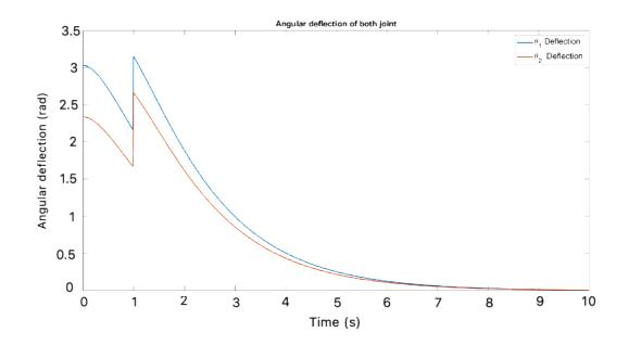
Figure 67: Angular deflection of both links of the simulated model with LQR controller
