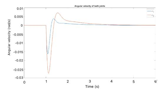
Figure 28: Angular velocity of both joints with LQR controller
