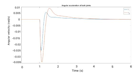
Figure 29: Angular acceleration of both joints with LQR controller
