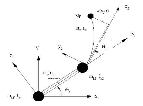
Figure 2: Rigid flexible manipulator
