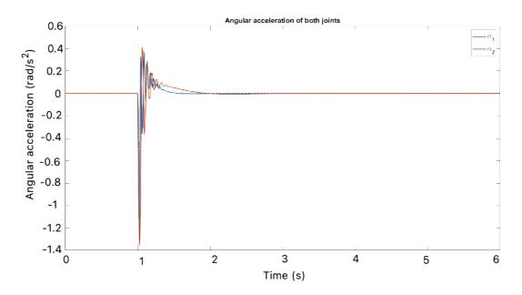
Figure 21: Angular acceleration of link 1 and link 2 with PID controller
