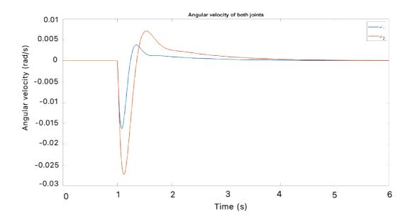
Figure 34: Angular velocity of both joints with LQG controller
