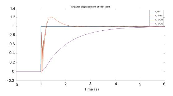
Figure 40: Comparison between angular displacement of link 1 for the three controllers
