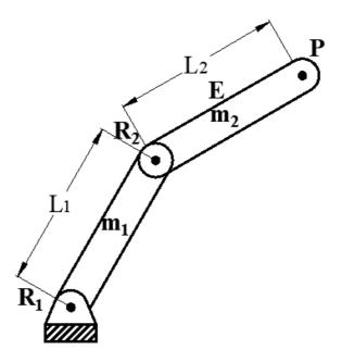
Figure 75: Free body diagram schematic for two-link manipulator
