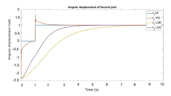
Figure 72: Angular displacement of link 2 of the simulated model with the three controllers
