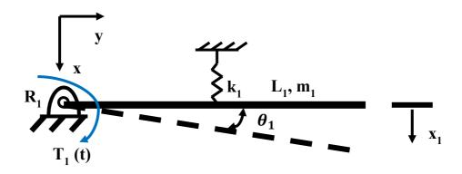
Figure 76: Link 1 schematic diagram
