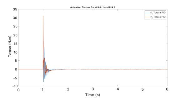
Figure 22: Actuation torque for both joints of manipulator with PID controller
