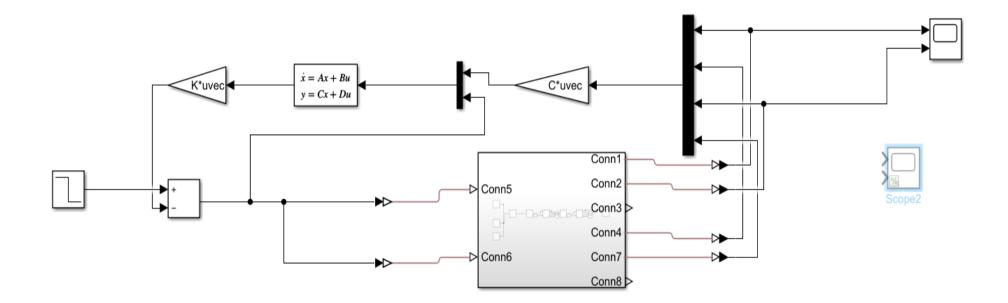
Figure 64: Simulink model of the LQG implemented controller in manipulator
