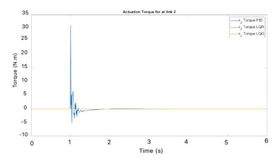
Figure 43: Comparison between actuation torque of link 2 for the three controllers
