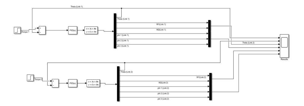
Figure 15: Model simulation using PID controller to track angular displacement
