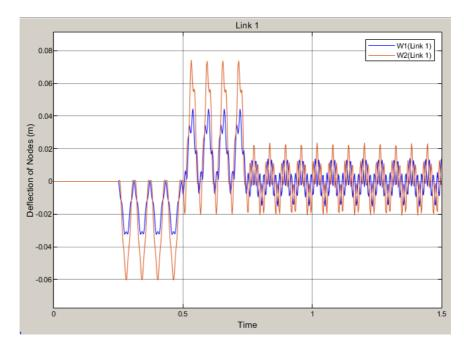
Figure 10: Deflection of nodes of link 1 without a controller
