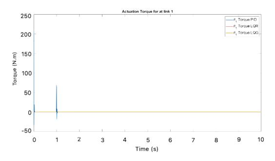
Figure 73: Actuation torque of link 1 of the simulated model with the three controllers
