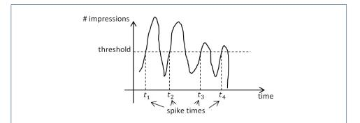
**Figure 6** Definition of spike time. As highlighted in the schematic, spike time is defined as the beginning of a series of impressions that exceed a certain threshold. In our analysis, the threshold is set to be the 95th percentile of the data.
