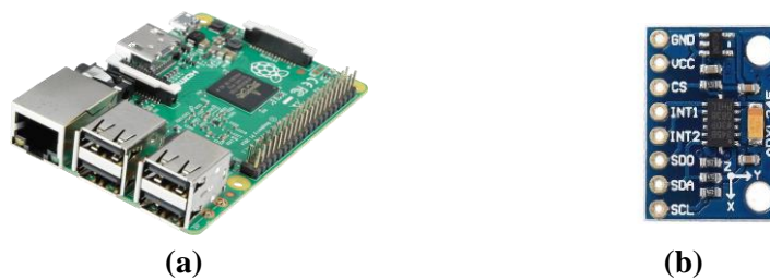
Figure 8. Hardware (a) Raspberry Pi 3 Model B+, (b) ADXL345 sensor
