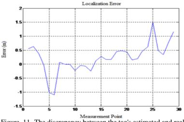
Figure. 11. The discrepancy between the tag's estimated and real range
