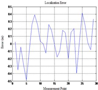
Fig. 9. Measurement error is the discrepancy between a tag's estimated and actual distance.
