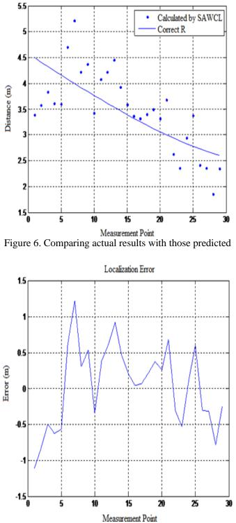
Figure. 7. Rotated power G-W403 tag error, calculated as he discrepancy between a calculated and a measured distance.
