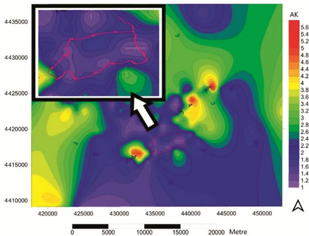
Fig. 7 — LRS route plan and soil amplification value (Av) map of the area
