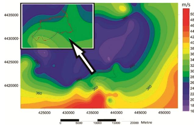
Fig. 5 — LRS route plan and  $V_{s30}$  map of the area
