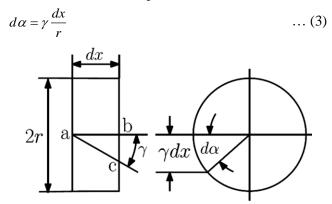
Fig. 3- Cross-section element of Spring.
