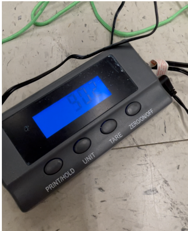
Figure 10: The scale showing a maximum force of 90.2 lbs
