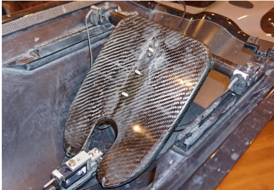
Figure 3: Foot Stretcher Force Sensor (Source: BioRow)
