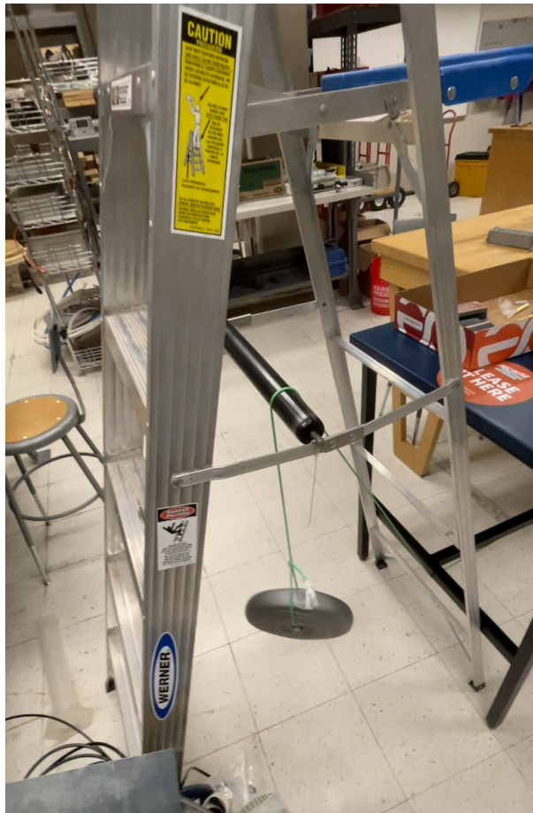
Figure 7: A ladder acting as a pulley for the 15 lb. weight
