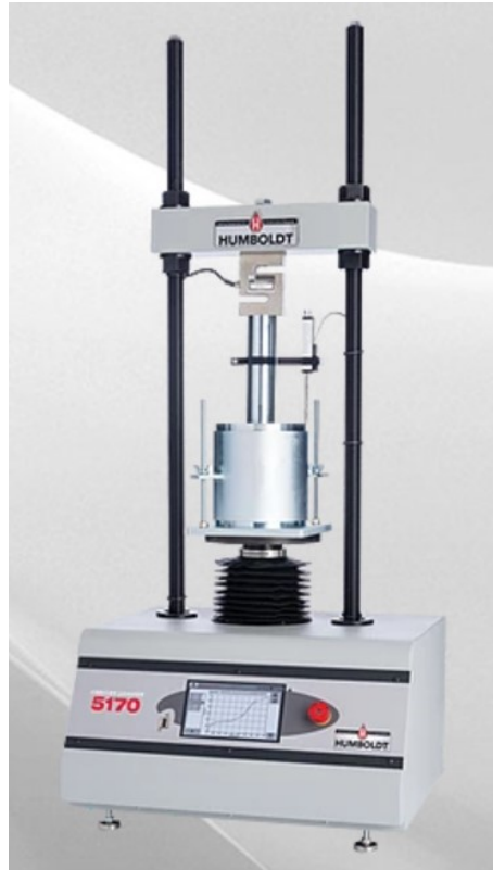
Figure 3: CBR/LBR and Marshall Automatic Load Frame (Source: Humboldt)
