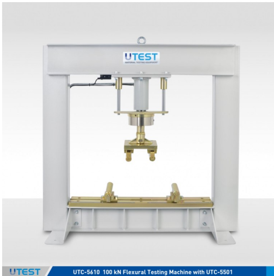
Figure 2: UTC-5610 Flexural Frame (Source: UTEST)
