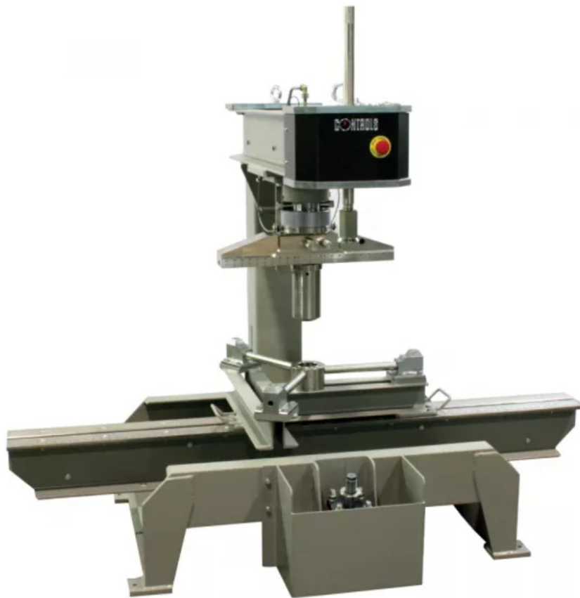
Figure 1: Uniflex 300 Flexural Frame (Source: Controls Group)
