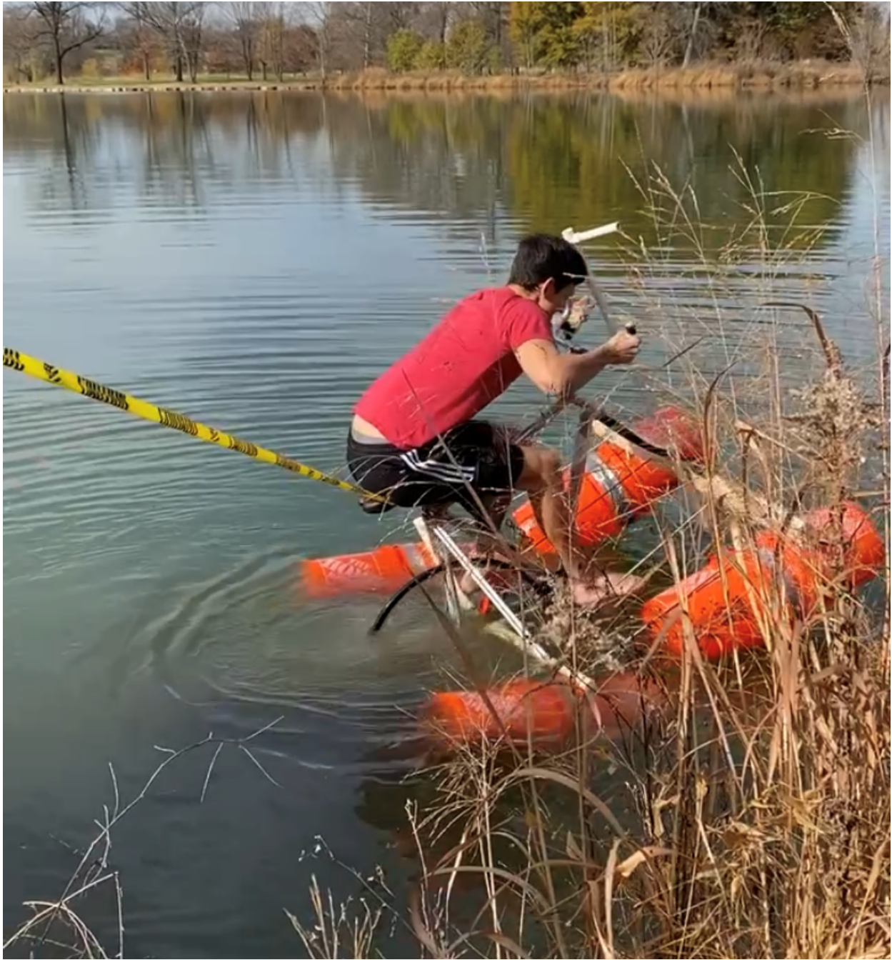
Figure 25: Water bike beginning to rotate backwards
