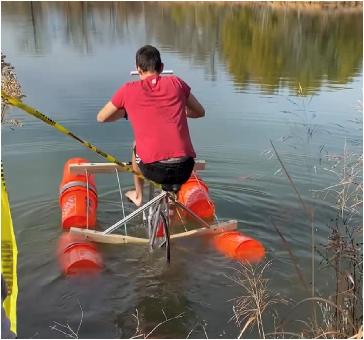
Figure 24: Water bike beginning to rotate backwards due to insufficient buoyancy in the rear pontoons
