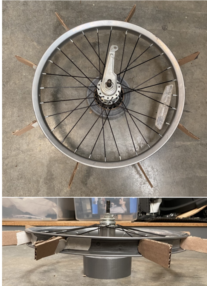
Figure 5: Top and Side Views of Paddle Wheel Mockup
