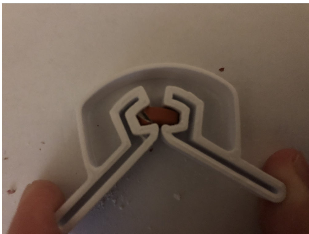
Figure 31: Shows crack propagation in the pill.
