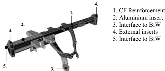
Figure 7 CDB mono-material parts
