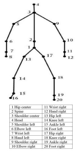
Fig. 3. Skeletal joints tracked by Kinect sensor
