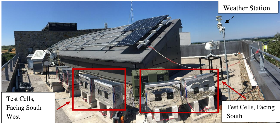
Figure 1. A labelled photograph of the outdoor experimental setup showing the eight test cells
