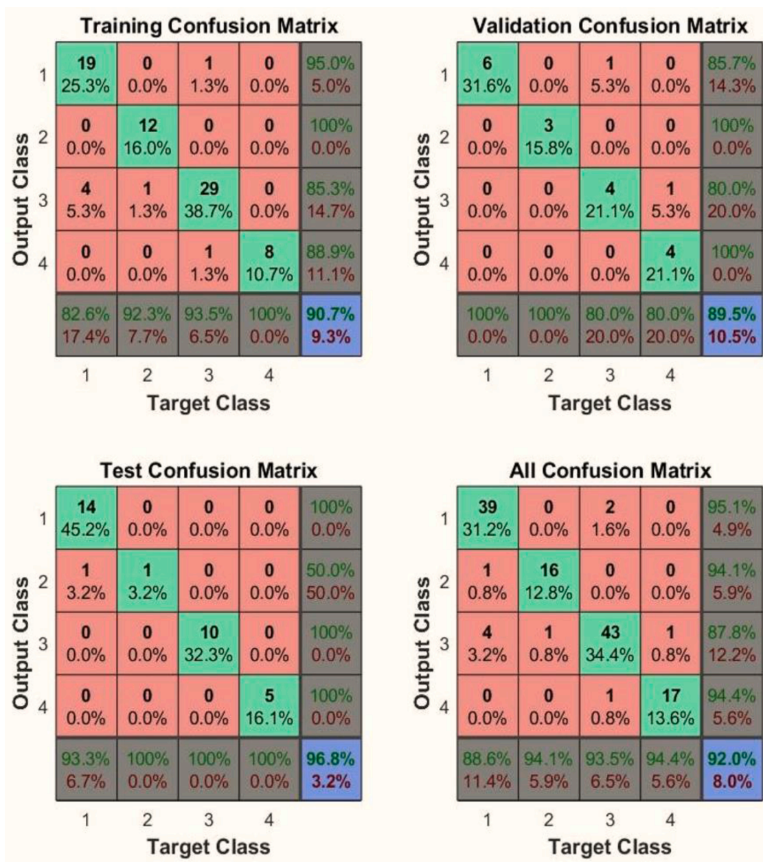
Fig. 14. Confusion plot of the DWT features applied in the combined neural network for flow regimes classification.
