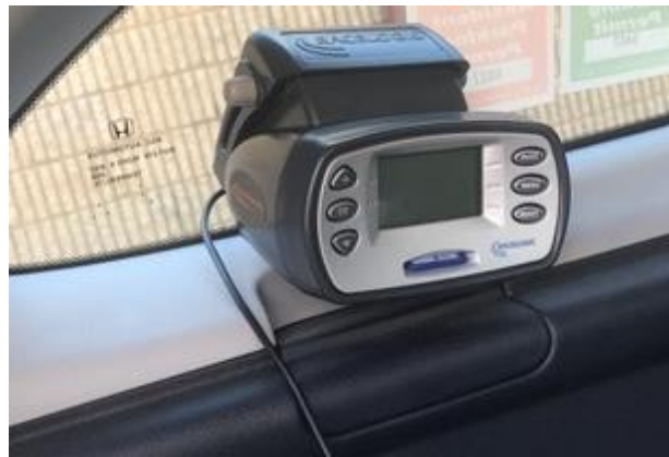
Figure 4.6 Performance-box installed on the window of tested car. (Photo credit by Yuanyuan Fan)
