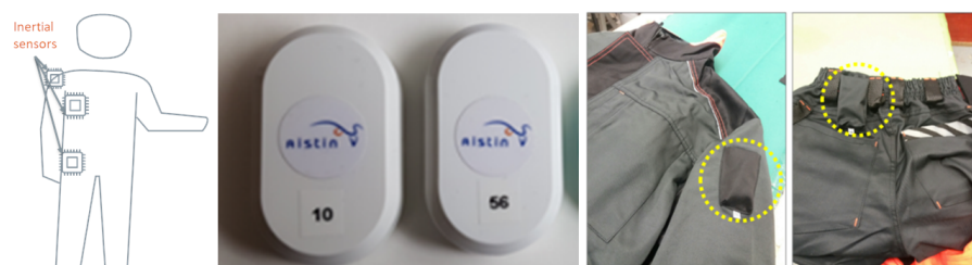
Figure 1. Depiction of the sensor locations. From left to right: planned locations, depiction of the actual sensors and example setup in the working clothes.
