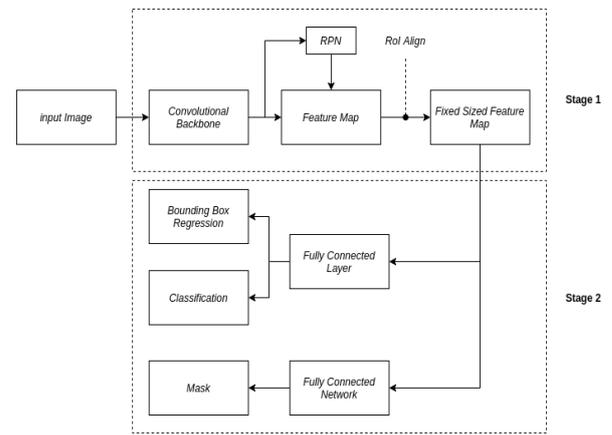
Gambar 8. Blok diagram alur mask R-CNN.
