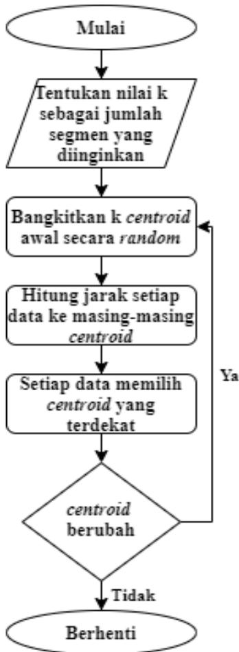
Gambar 1. Flowchart algoritma K-Means.
