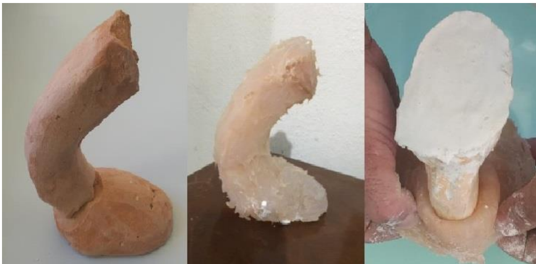
Figure 3 – Microscope 03 body preparation in clay (left), ready-made silicone mold (middle) and plaster cast being removed from the shape (right)
