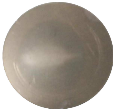
Figure 5.2.6: Target FL5 after two days of irradiation. The oval beam spot is clearly visible.
